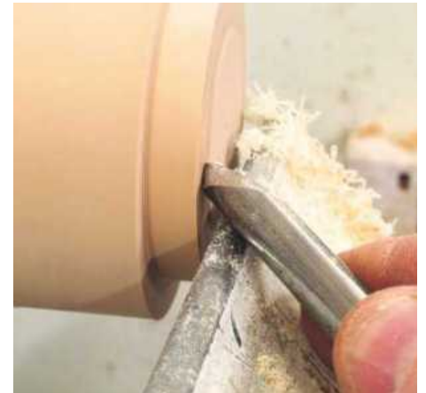
STEP 24. True up the face of the timber using a push cut from left to right, which will ensure there will be no tear-out on the outer edge. The lid then needs to be hollowed out and finished
